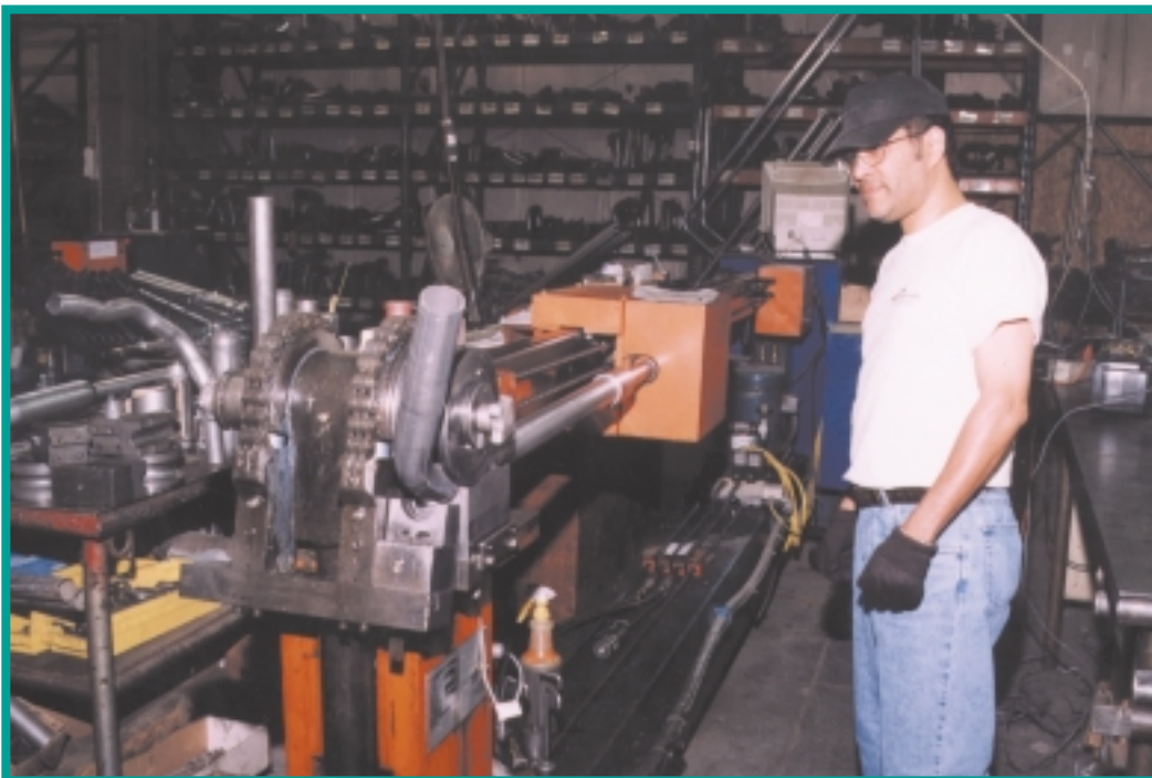
Jacques Fernandez bends a converter-assembly pipe with an upgraded Eaton-Leonard computerized bender. In the background are shelves full of assembly jigs used to guarantee proper fit.
