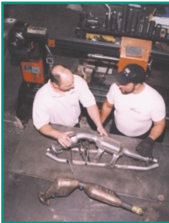
Bob Hamel (left) and John Medeiros check the fit of a Davico converter assembly. The replacement unit fits into the jig exactly the same as the OE unit in the foreground.
