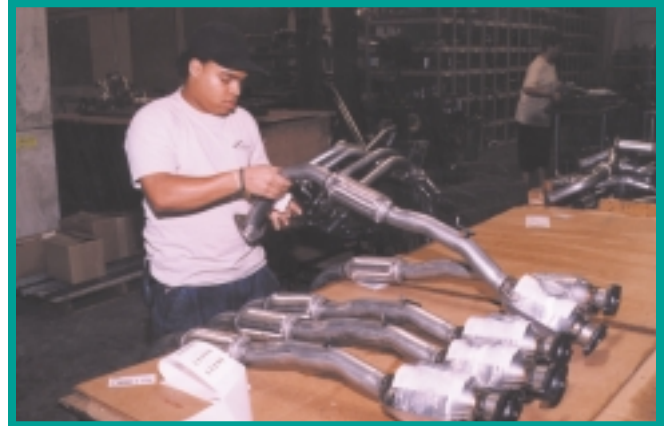
Edison DaCosta prepares converter assemblies, which include flex pipes, for shipping.
