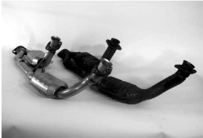
Making a replacement (left) for the original Ford Taurus catalytic converter (right), Davico did its usual flawless replication.
